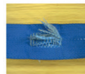
Any webbing which has been cut must be removed from service immediately.
