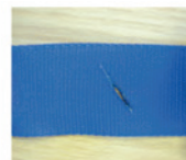
Webbing which has come into contact with hot material will melt and should be removed from service immediately.
