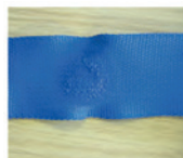
Webbing which has been exposed to elevated temperatures will stiffen and distort.
