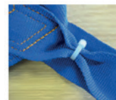
PPE must not be modified without approval by the manufacturer, any changes may affect the integrity or function of the item.
