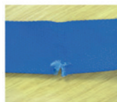
Nicks into load bearing webbing can lead to the webbing tearing across the weave when under load.
